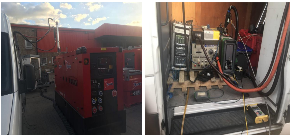
Fig. 2-1 Experimental setup - Analysing the exhaust gas emissions from a 100kVA ‘Speedy-Hire’ Generator using the ‘Emissions Analytics’ - Portable Emissions Measurement System (PEMS) Analysers - Semtech DS gaseous analyser and Pegasor Mi2 particulate matter analyser.
