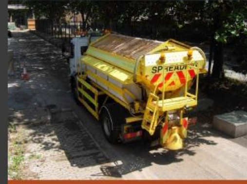
APPLYING CALCIUM MAGNESIUM ACETATE (CMA) AS A DUST SUPPRESSANT ALONG AN ON-SITE HAULAGE ROUTE
