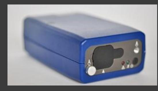
The **microAeth** is a self-contained, pocket-sized instrument with flow control, data storage, and battery and makes its analysis by collecting particulates on a replaceable filter strip and utilises the Aethalometer optical absorption technique to determine the mass concentration of Black Carbon in real time.
