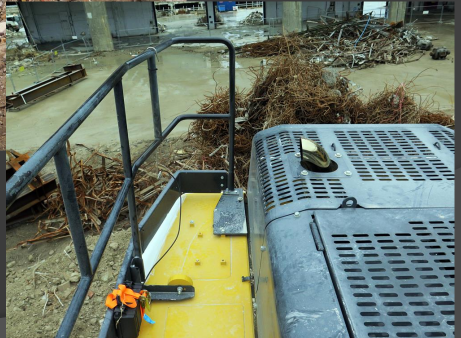
Komatsu PC 490 – 50t excavator EU Stage IIIB compliant Works in ‘isolation’ at high load to run hydraulics
