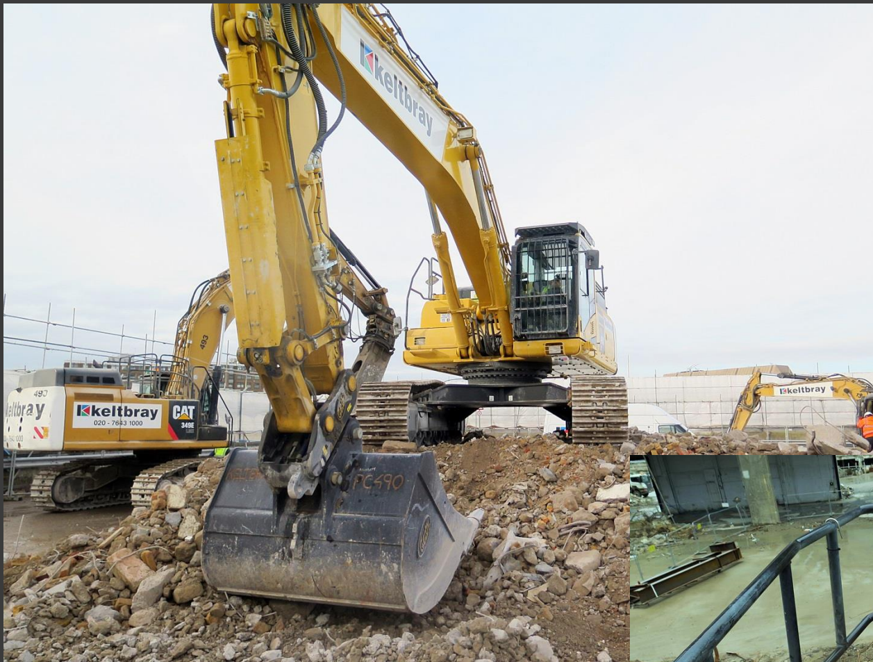
Komatsu PC 490 – 50t excavator EU Stage IIIB compliant Works in ‘isolation’ at high load to run hydraulics
